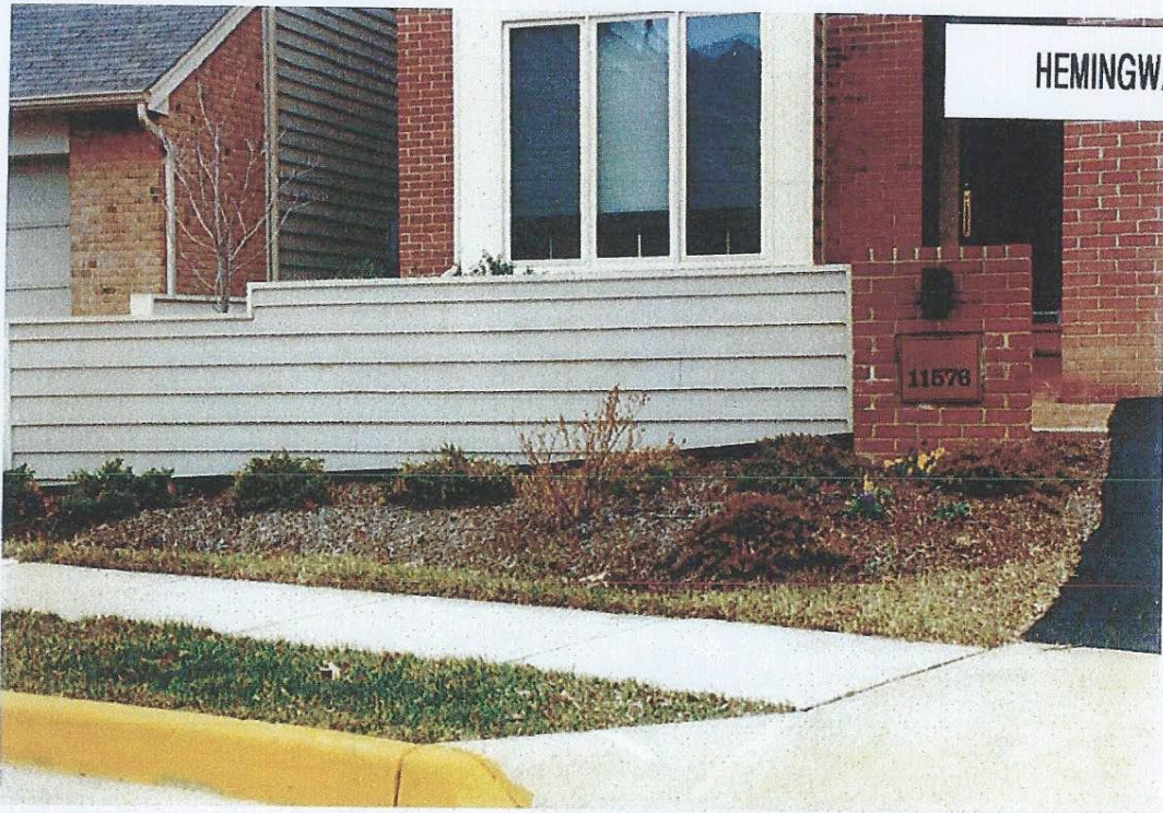
COURTYARD FENCE, Patio homes only (Same color, details, and materials as house siding. See specification sheet on reverse.)
